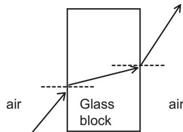
It is important to see that the ray bends towards the normal as it enters the more optically dense material, and away from the normal as it exits. Because the block has parallel sides, the incident and emergent rays are parallel.
