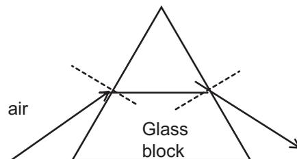
Again, the ray bends towards the normal as it enters the more optically dense material, and away from the normal as it exits. Because the block doesn't have parallel sides, the incident and emergent rays are not parallel.
